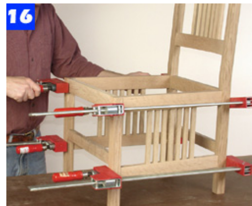
16 Join the front and rear leg assemblies to the side rails. Set the chair on a flat surface and clamp the joints.
