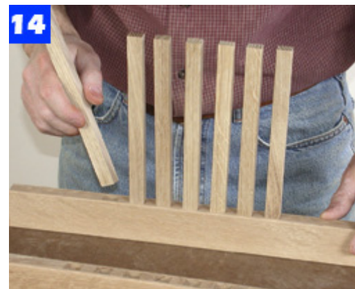
14 Install slats in the rails. You don't need glue unless the slats are too loose. Then add the remaining rails.
