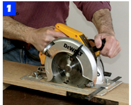
Use a circular saw and ripping guide to rip the stock. Clamp the work to your table so both hands control the saw.
