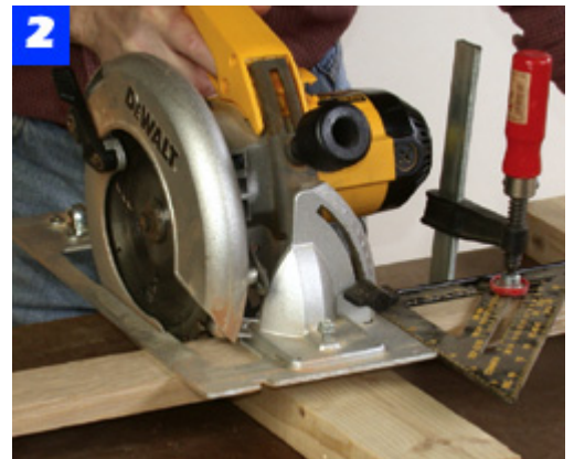
Clamp a speed square to the chair rail stock, and use it to guide the saw and ensure accurate crosscuts.
