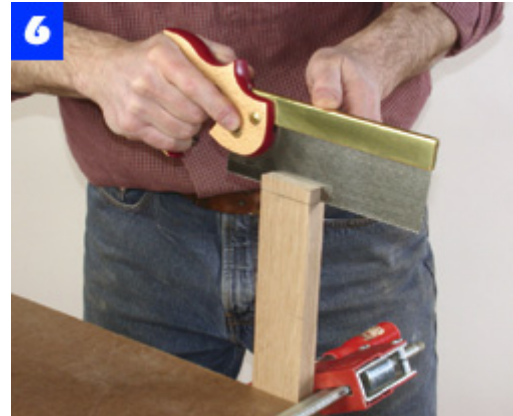
Clamp a chair rail to the side of your worktable and use a backsaw to make the tenon cheek cuts.
