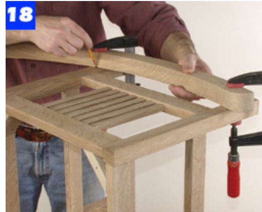
Clamp a rocker to the chair legs and mark the position of the rocker joint. Carefully cut the legs and test the fit.
