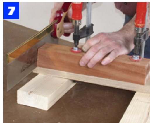
Make a guide by cutting the side-rail angle on 2-in. stock. Clamp it to the rail and hold the saw against its end.
