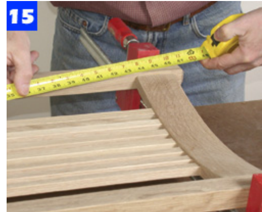
15 Spread glue and assemble the back frame. Clamp and compare diagonals to check that the assembly is square.
