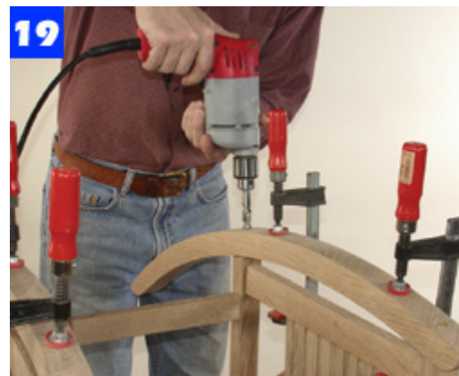
Clamp the rockers in place and bore a 1/2-in. hole through the rockers into the legs. Epoxy a dowel into each hole.
