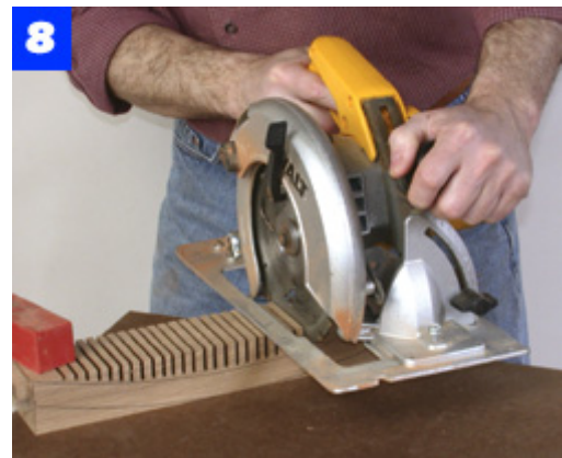
Use your circular saw to make a series of cuts that stop about 1/16 in. above the inside curve of each back rail.
