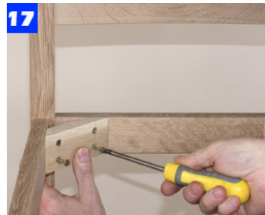
17 Cut corner blocks and countersink pilot holes. Install the blocks to the chair rails with 1-1/2-in. flathead screws.
