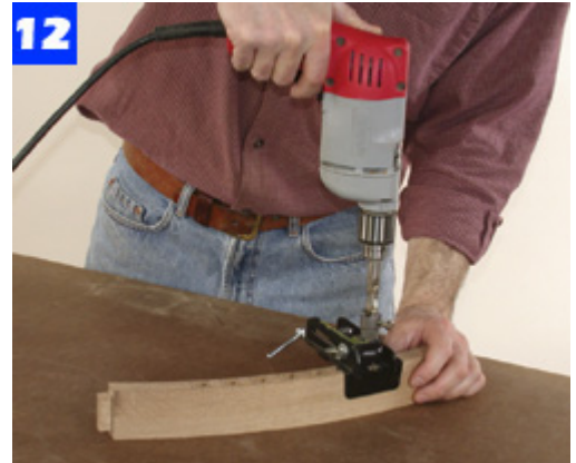
12 Use a 1/2-in.-dia. bit, doweling jig and depth stop to bore out most of the waste from each slat mortise.
